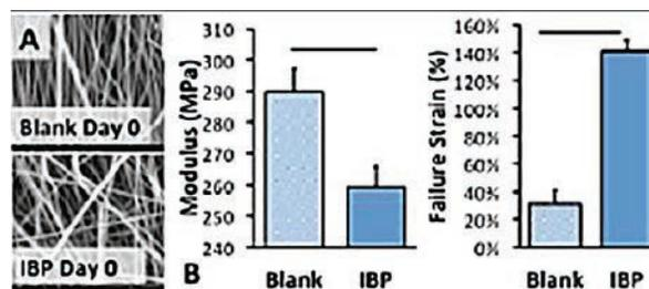
**Figure 3.** (A) SEM images of blank and IBP scaffolds prior to incubation. (B) Modulus and failure strain of IBP and blank scaffolds prior to incubation ( $p < 0.01$ ).
