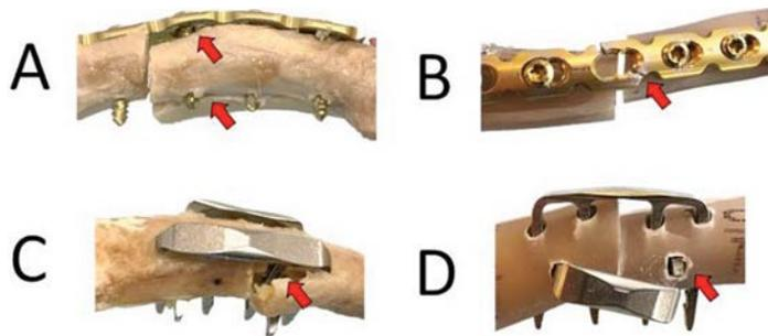
**Figure 3.** Differences in failure modes for cadaveric and synthetic specimens for the PLT and 2S groups.
