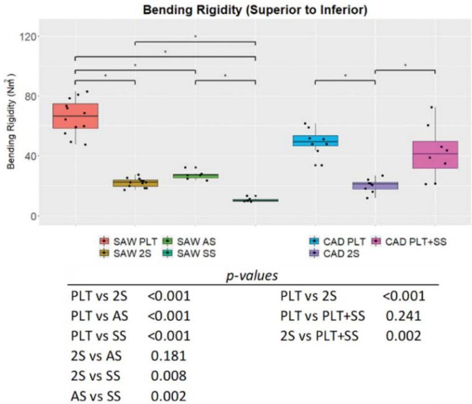
**Figure 2.** Results from non-destructive 4pt bend tests on Sawbones (SAW) and cadaveric (CAD) specimens.
