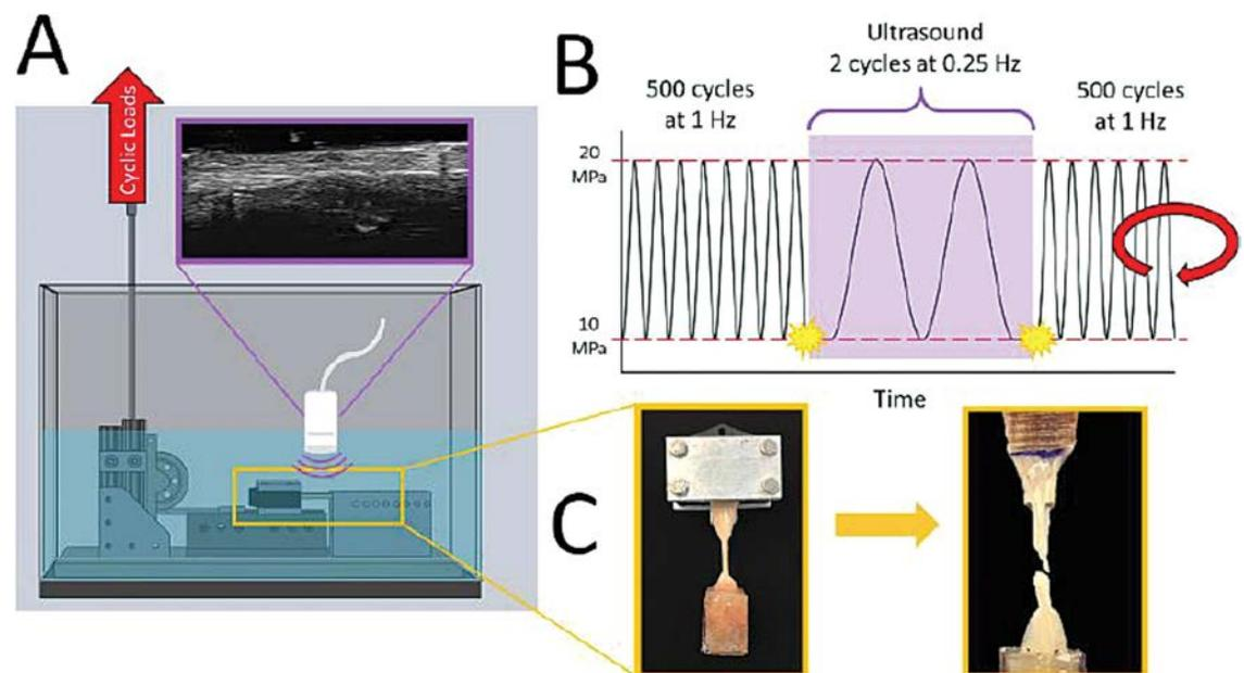
**Figure 1.** (A) Computer-aided representation of tank water bath testing setup, showing pulley, linear track, and tendon carriage setup. (B) Cyclic testing protocol applied to tendon. Ultrasound (purple) was captured every 500 cycles and initiated via a trigger signal (yellow bursts). (C) This protocol was repeated until tendon failure or until 150,000 cycles was achieved.
