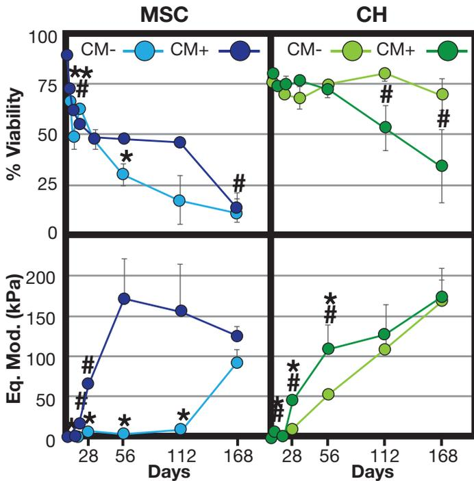
**Figure 1.** (Top) Viability in the center of constructs is less stable for MSCs, particularly at early time points ( $p < 0.05$ , \* vs. previous time point CM-, # vs. previous time point CM+). (Bottom) Eq. modulus of CH and MSC-laden constructs. ( $p < 0.05$ , \* vs. peak CM-, # vs. peak CM+).
