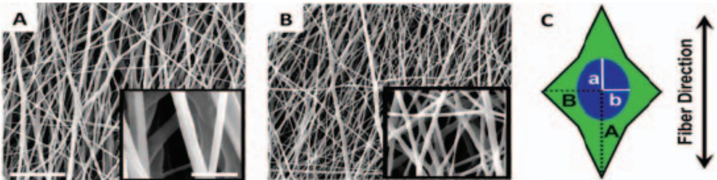
**Figure 1.** SEM images of large (A) and small scaffolds (B). (C) Schematic of cell measurements. Green is the projected cell area, CAR is the ratio of A/B, and NAR is the ratio of a/b. Scale = 10 μm. Inset scale = 2 μm.
